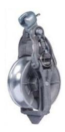
The DB7-H universal stringing block is made of 356 T6 aluminum alloy providing a 2,500lb safe working load and up to 2" diameter cable. Interchangeable with most common fittings and adapters for crossarms and insulators, the DB7-H has 90 degree mounts on the sides and underneath. Spring loaded gate opening allows for hotstick use with the ability to lock in the open position for easy removal of the conductor. Optional urethane lining available.
