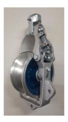
The STR-7 universal stringing block is made of A356-T6 aluminum alloy providing a 2,500lb safe working load and up to 2" diameter cable. Interchangeable with most common fittings and adapters for crossarms and insulators, the STR-7 has 90 degree mounts on the sides and underneath. Spring loaded gate opening allows for hotstick use with the ability to lock in the open position for easy removal of the conductor.
