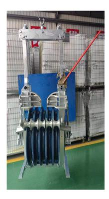
Heavy duty full frame block using steel framework, with A356-T6 aluminum alloy sheaves and UV resistant urethane lining. The center axle is 1045 steel by quenched and tempered heating. Optional Pac-Man style helicopter attachment available.
